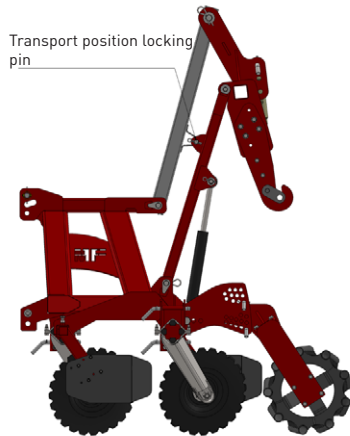
Fig. 11. Securing the cultivator in the transport position
